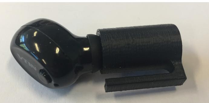
Fig 11 | Microphone attached to 3D-printed holder Author: Olivier van Duuren
